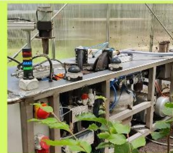
Semi-automatic device for the containerization of bare-rooted planting stock of trees and shrubs. Scan QR code above for demo video.
