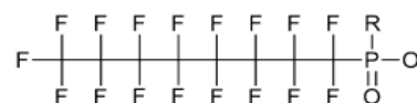
Perfluorophosphonic/phosphinic acids (ex. If R=OH then PFOPA If R=C8 perfluoroalkane then 8:8 PFPi)
